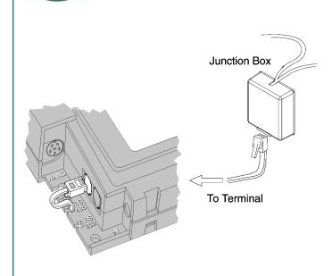
Make sure the power is off at both the time clock terminal and the PC, and the access door on the terminal is removed.
